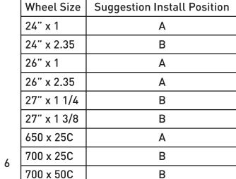
**Position A 3.** The Giant Cyclotron Mag trainer provides two resistance unit mounting locations to accommodate resistance unit, check the wheel size of your bicycle
