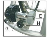
tire for the manufacturer's recommended pressure range, and inflate accordingly. Using the Adjustment Knob "G" set the Magnetic Resistance Unit "H" so that the roller contacts the bike's rear tire. Then turn the Adjustment Knob "G" clockwise two full turns to insure that you have sufficient pressure of the Drive Roller "E" on the rear tire.
