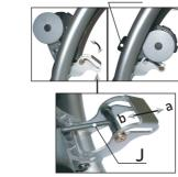
Adjustment Knob **"G"**. Try to move linkage pillar from frame attachment stay tracking location (a) to (b) until it's locked.
